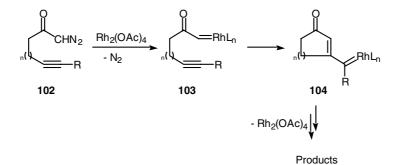
The reaction is believed to proceed via decomposition of the  $\alpha$ -diazo ketone **102** to generate a rhodium carbenoid intermediate **103**. Addition of the rhodium-stabilised carbenoid onto the alkyne  $\pi$ -bond generates a vinyl carbenoid intermediate **104**, in which carbene-like character has been transferred to the more remote carbon of the alkyne. The intermediate vinyl carbenoid may then react further in either an intra- or intermolecular fashion to give novel products.
