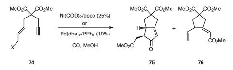
$\alpha$ -Methylenecyclopentenones, fused to five-membered rings, have also been prepared via a palladium-catalysed (10 mol%) carbonylative cyclisation (40–100 atm carbon monoxide) of enynes [70].
